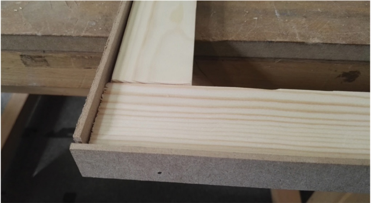
MDF sections are cut deeper than the depth of the strainer bars. This ensures that the canvas sits above the frame
