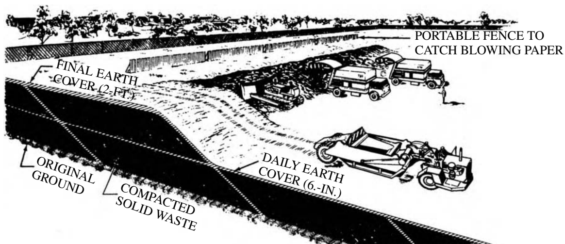
FIGURE 13 Area method. The bulldozer spreads and compacts solid wastes. The scraper (foreground) is used to haul the cover material at the end of the day's operations. Note the portable fence that catches any blowing debris. This is used with any landfill method.
