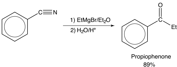
Figure 10-13: Using a Grignard reagent to convert a nitrile to a ketone.
