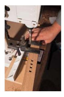
The best method for mortising is to first bore the areas at either end of the mortise, then space the next few mortises the width of the mortising chisel. In this case, the spacing works almost perfectly. The goal is to allow the chisel bit to have enough wood to drill straight without wandering from side-to-side. On some mortises the spacing between the first holes will be less than the width of the chisel.
