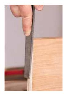
To trim the long edges of the veneer tape, the tool of choice is a mill bastard file. Start by flushing the ends you just broke over, keeping the file flat to the side, and using only a pushing stroke. It should only take a couple strokes to flush up the end.
