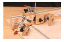
HOLD IT The hold-downs and stops are made from 3/4" hardwood. To make the guide to hold the stops square to the fence, cut a 1/16" x 1-1/8" rabbet on both sides of the inside face.
