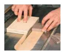
Wedges The wedges are cut on the table saw using a simple jig (see diagram below). The stock is ¾" x 6" x 3". That means the grain direction is in the 3" dimension. Make a simple jig to hold the wedge stock while cutting on the saw.
