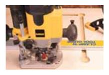
ROUT THE GROOVE The grooves for the T-slot track allow the fence to be used left-to-right and front-to-back on the table to take advantage of the built-in tilting feature of the existing table.
