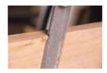
To trim the tape edges, use the file again, working right to left against the edge. The best method is to start the file at the end of the tape and push lightly against the overhanging edge to start a curl of veneer breaking away from the edge. Continue rolling the curl along the piece, keeping the file angled forward and at a slight bevel to the veneer tape. Once the curl is knocked off, lightly file the bevel again to remove any excess.
