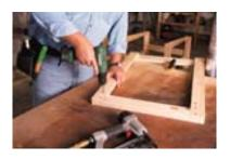
As you can see on the end, the back stiles are glued together to form "L"-shaped sides, then the back rails are screwed in place between the two sides. The 1-½" rail is attached to the upper rail to make a more solid looking and feeling back.
