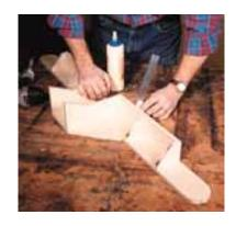
As you assemble the fence, make sure it is square along its length. Be sure and check it again after it is clamped up.
