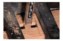
Complete the mortise by drilling away the waste between the first mortises. This allows the mortise chisel to cut most efficiently without pulling to the left or right and bending the chisel.
