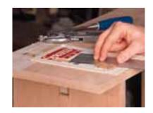
Trimming Tenons When the glue is dry and cleaned up, make a template out of the cover from a steno pad. The front and back will do. Just tape them together and cut out a couple of holes for the tenons to come through. The more difficult set of tenons to reach are the ones below the top. Set your template up for those. Lay the template over the tenons and cut them flush with the template.
