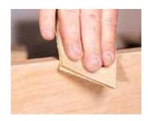
The file is too aggressive for a finished edge, so trade it in for some 220-grit sandpaper and finish cleaning up the edge. You'll find some of the adhesive is stuck to the face of the board. This can be lightly sanded off, but proceed carefully to avoid sanding through the face veneer. That's all there is to it, but don't go using the clothes iron, buy your own for the shop!
