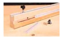
tracks in the grooves with flat head screws countersunk into the track. The braces are attached to the fence by screwing through the face groove prior to attaching the T-slot track.
