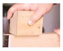
Since trying to use the iron to hold the tape in place as the glue dries just re-heats the glue, switch to a simple block of wood. The chunk of poplar shown here works great. The bottom surface is sanded smooth and the edges are broken to avoid snagging or scratching. Simply apply pressure and make long passes over the edge for about 30 seconds. If you have a few pieces to veneer, set the first piece aside for now to let the glue cool.
