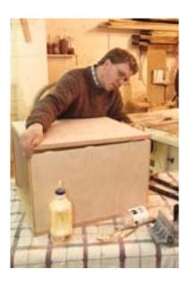
During the second stage of cabinet assembly, laying the cabinet on its side keeps you from fighting with gravity. The cabinet comes together relatively easily, and the alignment is a snap thanks to the biscuits.
