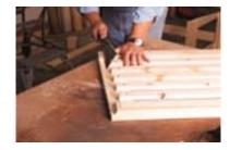
With the back slats in place, the ends of the back stiles need to be beveled to allow the back to recline to a comfortable position. I'm beveling the pieces here with a pull saw at more of an angle than necessary, but it won't hurt anything.
