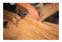
After you cut your tenons, lay them directly on your work and use the edges like a ruler to mark where the mortise should start and end (this picture).
