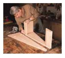
With all the cross members cut, the biscuit joiner makes it possible to pull the project together. This photo also shows the two cleats in place at the top and bottom of the case.
