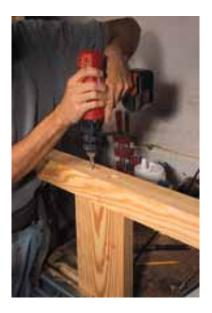
Drilling the 3/8" holes for the bolts is easier if you do it in this order. First drill the holes in the legs using your drill press. Now assemble the leg and front rail. Drill into the rail using the hole in the leg as a guide. Remove the leg from the rail and continue drilling the hole in the rail. The hole you drilled before will once more act as a guide. You still need to be careful and guide your drill straight and true.
