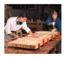
When you glue up your top, you want to make sure all the boards line up. Lay down your glue and then clamp up one end with the boards perfectly flush. Then get a friend to clamp a handscrew on the seam and twist until the boards are flush. Continue clamping up towards your friend, having your friend adjust the handscrews as needed after each clamp is cinched down.
