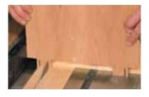
Cutting Tenons Cut the tenons to the actual width on the table saw. Set the blade to 1" high, defining the length of the tenons. After marking the depth with a gauge, cut the waste out from between the tenons. Set the saw to 7/8" high for cutting the slots that accept the wedges used to hold the table together. See the diagram for the actual size of the outer parts of the tenon. Use a backing board on your miter gauge to hold the boards upright.
