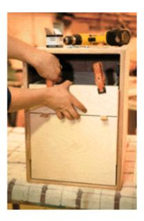
A consistent reveal is key to the crisp feel of the piece. The shims shouldn't bow the cabinet sides out at all, but should fit snugly to ensure that the drawer front is centered and that the reveal is even on both sides.
