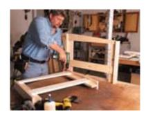
With the legs assembled, attach both lower side stretchers. Then place an upper stretcher in position and draw a line from the top of the angle on the back leg to the front leg. Cut the stretcher on the mark, then attach the upper stretchers, completing the two side frames.
