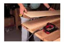
Face-Glue the Parts: Once you've got your parts cut to size, glue and nail them together leaving the rabbet at the back. Set and putty the nails, then rip the dividers to their final width.
