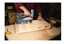
This shot shows the partially assembled table, with three exposed dividers and the other side covered with the top. You can also see the screws through the bottom that hold the mounting blocks in place. While the box itself is nailed together, the fence is attached with screws to allow for replacement if it gets cut up too much in use.
