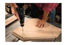
wood should be as long as your table saw's fence. Its width depends on how thick your project's stock is. For cutting patterns in ¾" stock, rip this board to 1-5/8" wide. The second one should be 1-¾" wide and about 6" shorter than the first board. Nail and glue these two boards together using the drawing as a guide.
