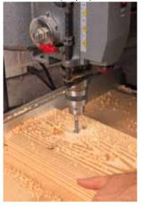
The mortises in the front rails are also made on the drill press. Make them 1-1/4" deep to make sure you can get a washer in there. If you can't, try clipping an edge off of the washer.
