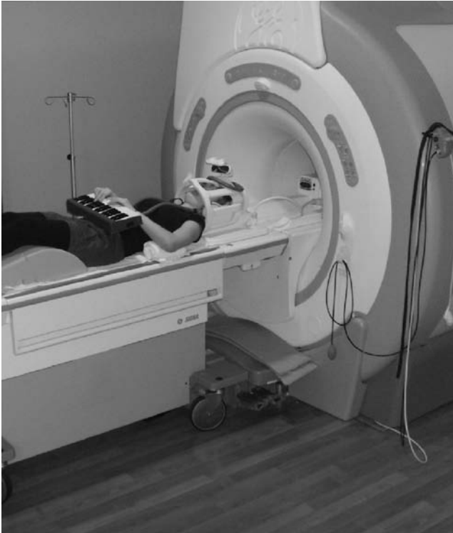
Figure 4.4 Experimental participant with keyboard, preparing for an fMRI experiment concerning music performance. Prior to the experimental session the participant will be moved back so that her head sits within the bore of the scanner.
