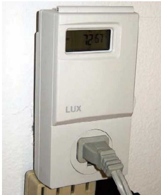
A digital thermostat controlled switch is used for cooling or heating the grow room
