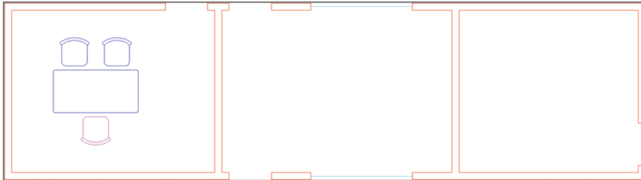
FIGURE 7.18 Turning off the Door layer hides the doors but not the chairs when the chair block definition geometry is on layer 0.
