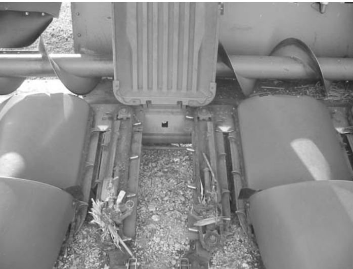
Figure 5.3 Gathering chains and stripper plates over stalk rolls (middle snout is raised).
