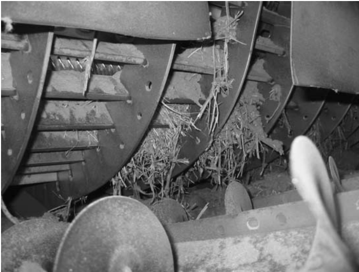
Figure 5.6 Rear of concave underneath cylinder (note clean grain augers underneath in foreground).
