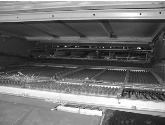
Figure 5.10 Top sieve (chaffer) in cleaning shoe as viewed from rear of combine.
