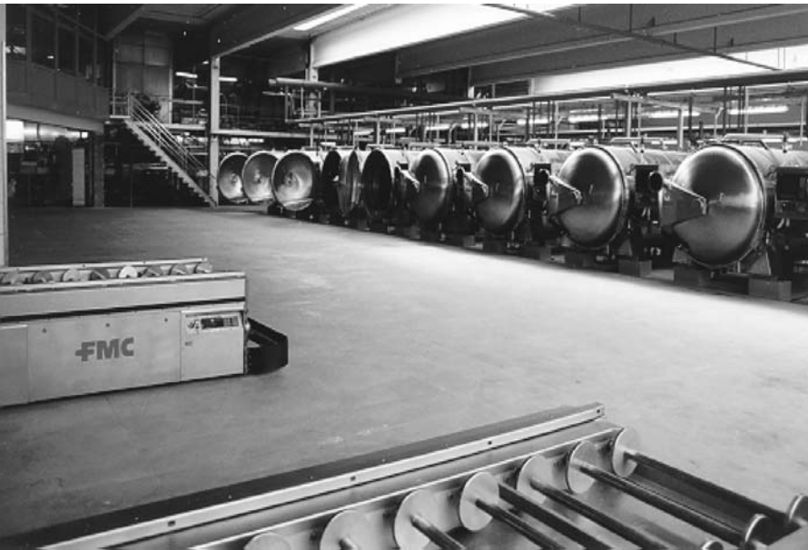
Figure 15.7b Batch retort system in large cook-room operation (courtesy of the FMC Corporation).
