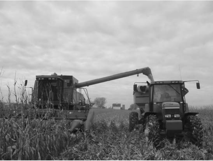
Figure 5.13 Unloading auger extending and moving grain to transport cart.
