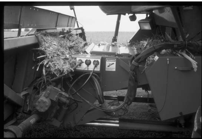
Figure 5.4 Feederhouse connecting head to combine threshing area.
