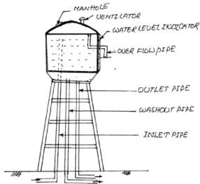
Fig 8.5. Overhead Tank
