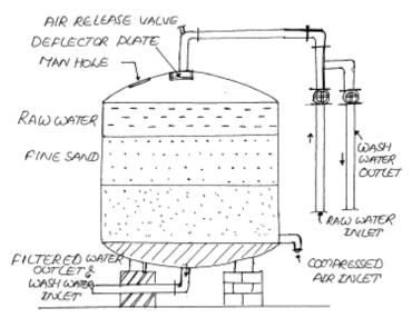
Figure 5.6 Vertical Pressure Filter
