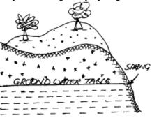
Fig 3.5 Gravity Spring
