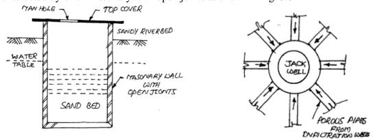
Fig 3.3 Infiltration Well
