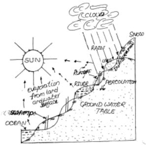
Fig 3.1 Hydrological cycle
