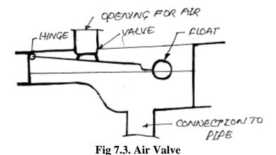
This valve consists of a chamber in which one or two floats are placed and is connected to the pipe line. When there is flow under pressure in the pipeline water occupies the float chamber and makes the float to close the outlet. But where there is accumulation of air in the pipeline, air enters the chamber, makes the float to come down, thus opening the outlet. The accumulated air is driven out through the outlet.
