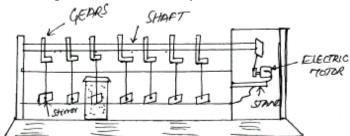
Fig 5.2 Jar Test Apparatus
