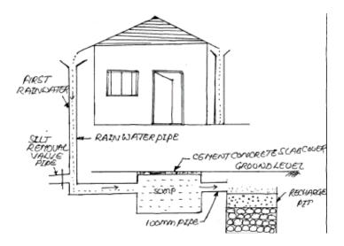
Fig 9.1 Storage Sump and Recharge Pit
