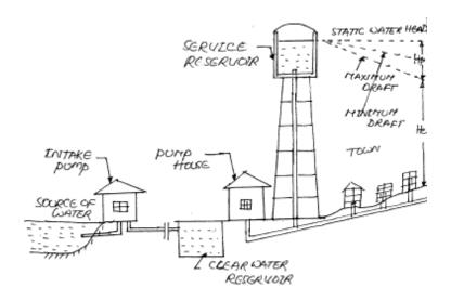
FIG 6.7 Dual System of Distribution
