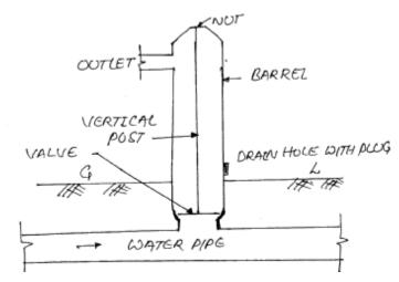
Fig 7.4 POST FIRE HYDRANT
