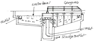
Fig 5.2 Sedimention with Caogulation
