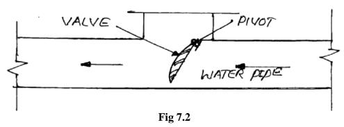
When the water moves in the direction of arrow, the valve swings or rotates around the pivot and it is kept in open position due to the pressure of water. When the flow of water in this direction ceases, the water tries to flow in a backward direction. But this valve prevents passage of water in the reverse direction.
