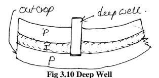
The depth of deep well should be decided in such a way that the location of out crop is not very near to the site of well. The water available at a pressure greater atmospheric pressure, therefore deep wells are also reffered to as a pressure wells.
