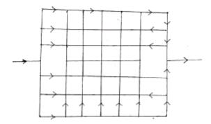
Fig 6.3 Circular of Ring System
