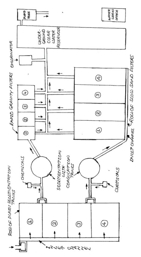
Fig 5.1 Typical Layout of water treatment works
