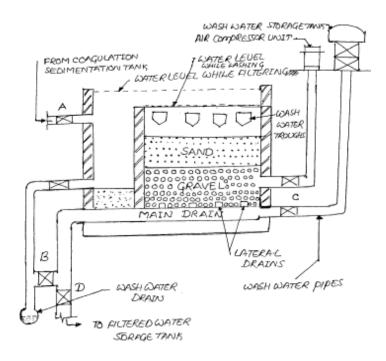
Fig 5.5 Rapid Sand Filter
