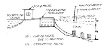
FIG 6.5 Gravity System
