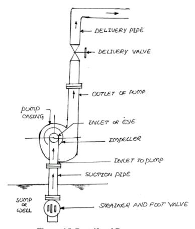
Figure 6.8 Centrifugal Pump
