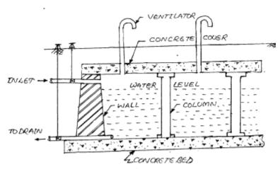
Fig 8.6. Under Ground Reservoir
