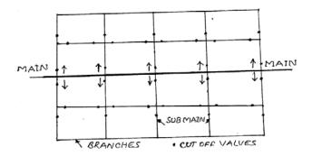
Fig 6.2 Grid – Iron Method
