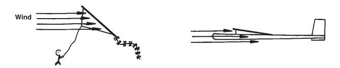
Our glider flies because of this angle of attack into the wind, this known as the angle of incidence.
