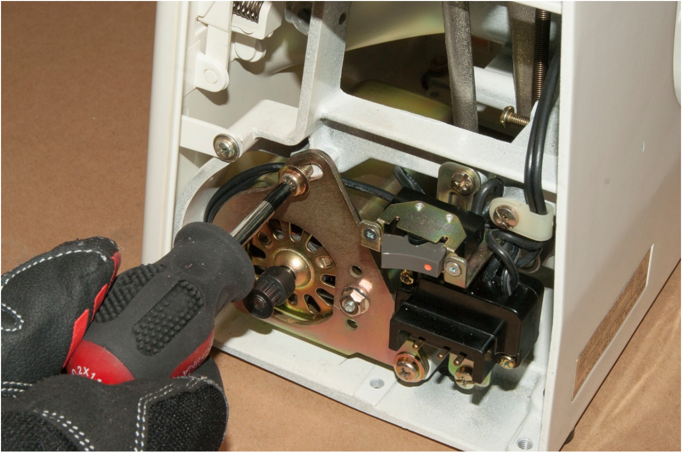
Install the new drive motor.
