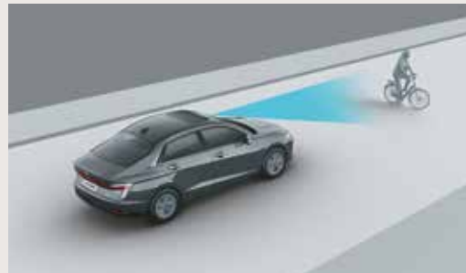
Forward Collision - Avoidance Assist - Cycle (FCA-Cyl)
