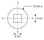
(i) Moment of inertia of solid circular section about x-x axis
